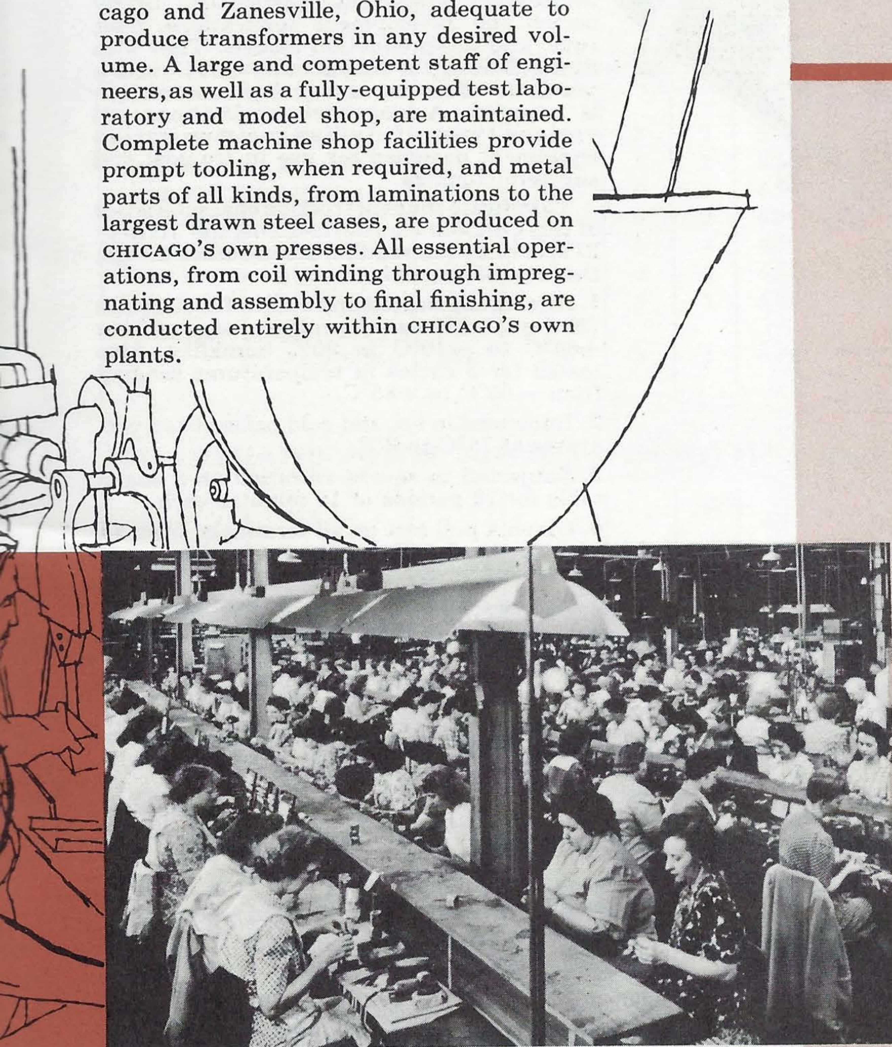
One of several CHICAGO assembly departments. Here, insulated leads are attached to the coil, and laminations inserted around the coil to form the core
