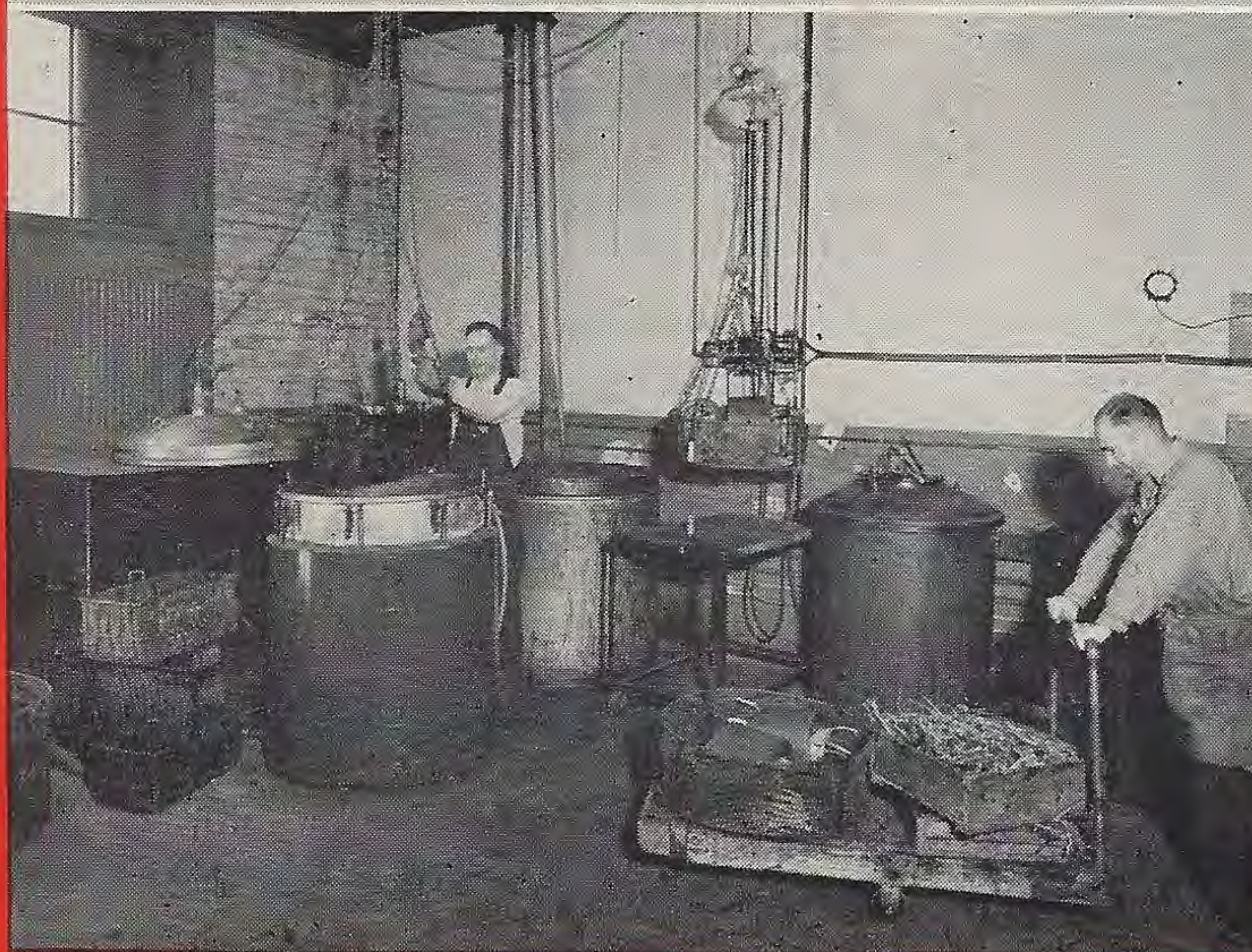
Series of vacuum impregnating tanks where the transformers go through Peerless's exclusive Vac-Seal process. Center is an electric baking oven; left and right are vacuum tanks.
