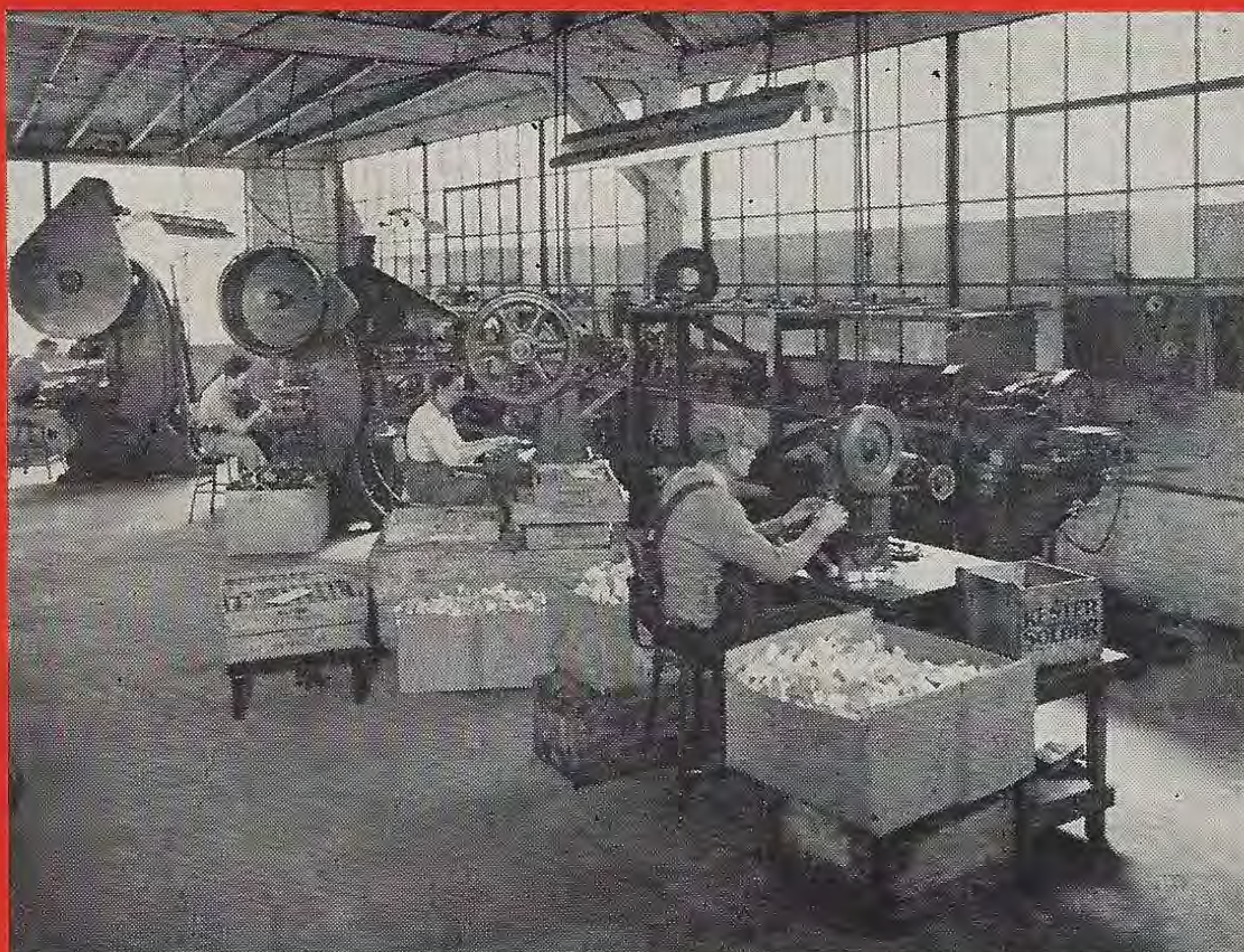
A corner of the stamping department. Punch press operators are forming Peerless transformer cases. In the background are dies for making laminations and various sized cases.
