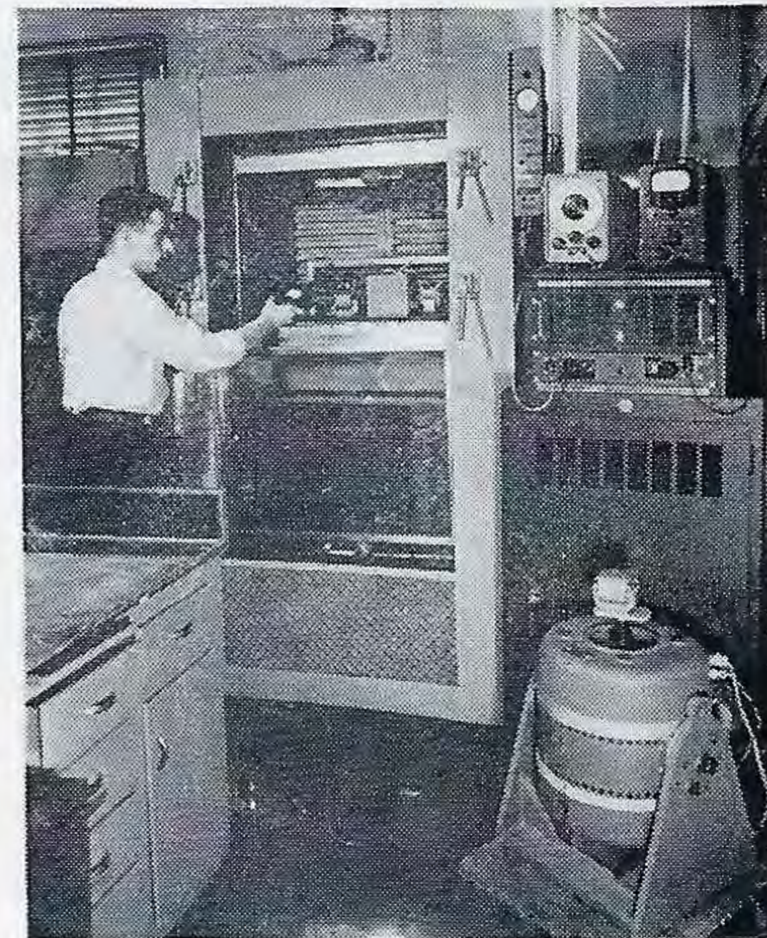
Altitude Test and High Frequency Vibration for Airborne Units
