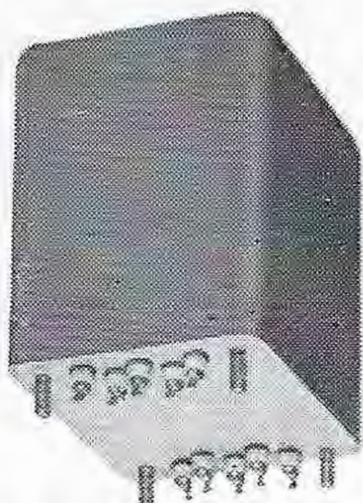
Magamp for 50 watt, 60 cycle servomotor. Two control windings. One feedback winding, one power winding, diode panel. Power gain 100. MIL-T-27A; 30 lbs.
