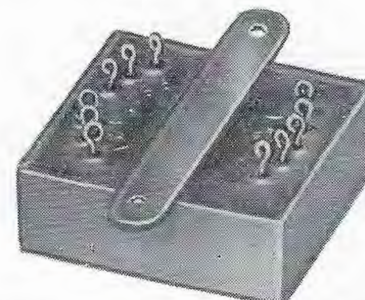
Instrument reference transformer. Input 50 V. 400 cycles. Three 5 V.-.025A. Outputs to .05% accuracy. Saturation characteristics and DCR balance to 3%. MIL-T-27A; 1½ x 1¾ x ¾, 2 oz.
