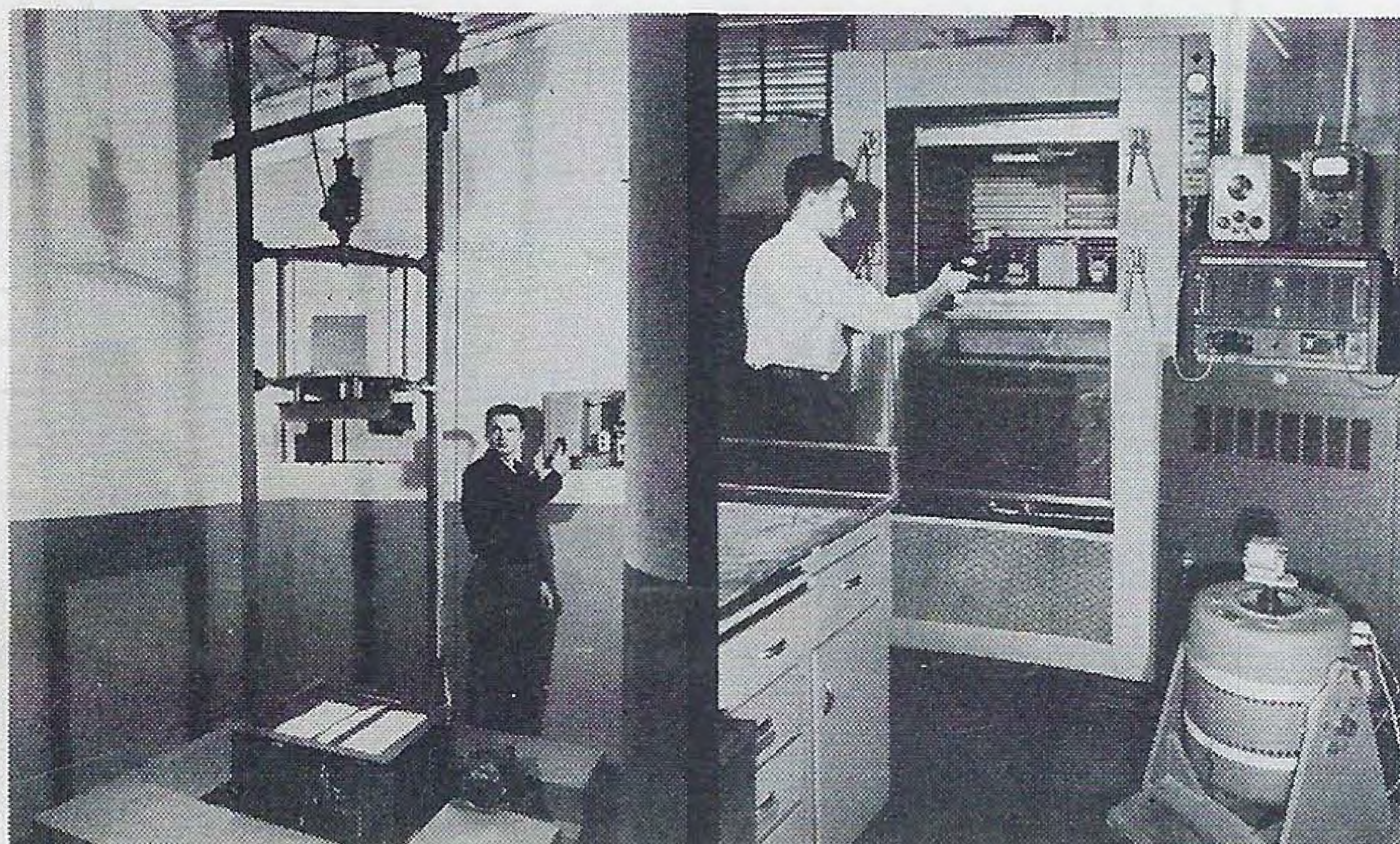
Altitude Test and High Frequency Vibration for Airborne Units
